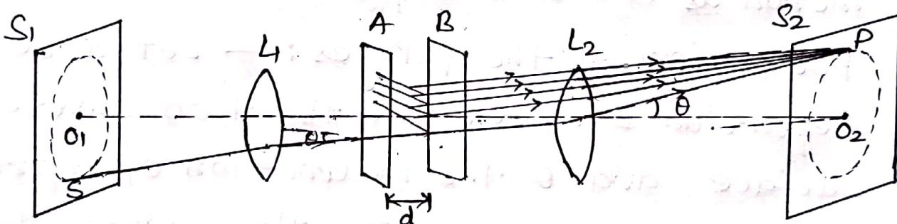
It consists of two optically plane glass plate A and B with their inner surface silvered, and placed accurately parallel to each other. Screws are provided to secure  $\Rightarrow$  parallelism if disturbed. The plate themselves are slightly prismatic to avoid interference among the rays reflected at the outer unsilvered surface.
